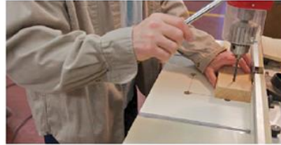
It's dangerous to wear loose, untucked clothing or long, unbuttoned sleeves when working around moving machinery parts.
