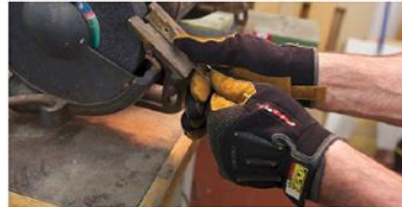
Even close-fitting gloves can get caught by moving machinery parts.
