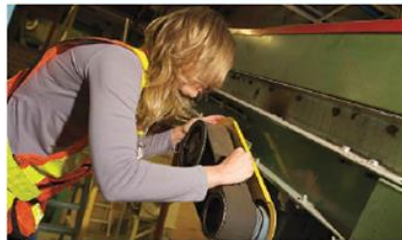
Hair that is long and loose can create a hazard. Tie back or cover long hair and facial hair when you're working around moving machinery parts.
