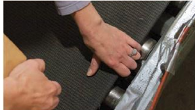
Rings and other jewellery are easily caught by moving machinery parts. Do not wear jewellery at work.
